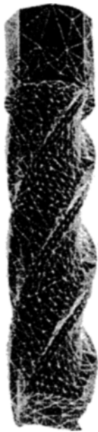
Fig. 6 Mesh generation for tool deflection calculation by FEM.
